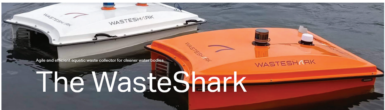
Figure 3. The WasteShark autonomous surface vessel for aquatic waste collection (RanMarine Technology, 2025).
